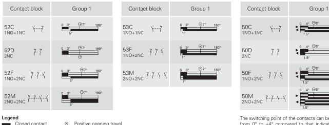
The switching point of the contacts can be adjusted from 0° to +4° compared to that indicated in the travel diagrams. The hinge is supplied without preadjustment.
